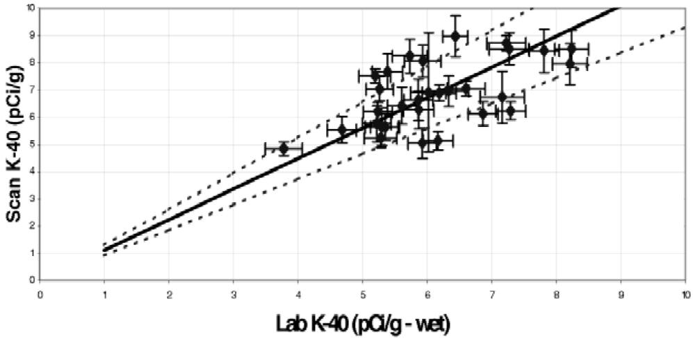
Fig. 3. Comparison between K-40 results from soil sampling and from the scanning spectrometer system. (Paper 3)
