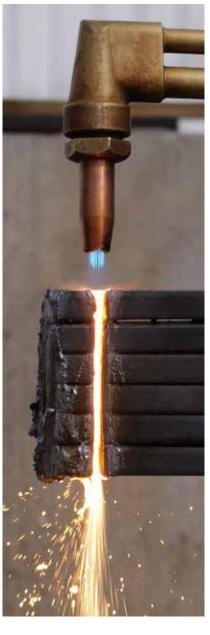
heavy vapors of liquid fuel's push combustion all the way down the length of the flame. This longer duration of combustion pushes further into the steel and continues to heat down the length of the steel. The BTUs released by the burning steel also add to the flame's heat and penetration.
